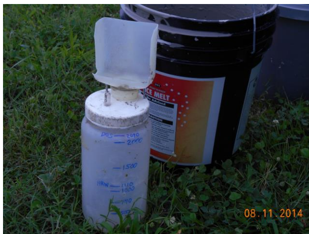
(4a) (4b) Figure 4. HRW applicator (a) and HRW on grass in plot after application (b).
