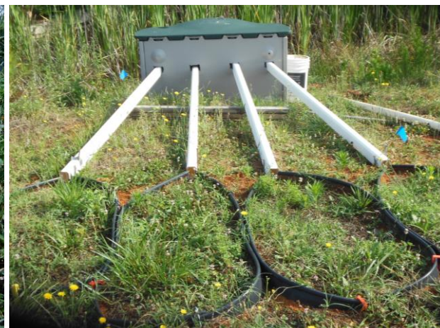
(3a) Figure 3. Field plot vegetation (a) and runoff collection system (b).
